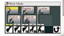
When replacing the attachment, oil flow adjustment can automatically be done by one touch on the work mode selection display on the LCD monitor. Minor adjustments of oil flow is possible if necessary.
