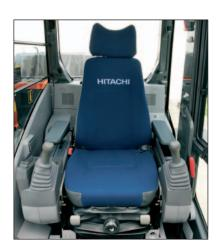
Wide adjustable armrests and a retractable seat belt are included. Short stroke levers mean fingertip control of hydraulics and allow for continuous operation with less fatigue. Three switches on the lever (optional) can be set to operate attachments other than buckets. The cab is pressurized to keep out dust. Noise and vibrations are kept to a minimum due to the elastic mounts, filled with silicone oil, the cab rests on.
