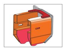
The idler bracket reinforcing plate is thickened greatly for higher durability to prevent the opening of idler bracket. The track link disengagement preventive plate, located just behind the idler bracket, is thickened for higher durability, and reshaped by extending its stepped end to prevent the disengagement of track links.
