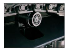
The X-beam is strengthened by the improved construction and enlarged box sections. The section is increased in strength up to 35%. Top and bottom plates of the X-beam use monolithic plates, instead of conventional welded four plates. This eliminates welding to strengthen the X-beam. Upper and lower rollers and upper roller brackets are increased in size for higher durability. Track links are thickened and reshaped for higher durability and rigidity.
